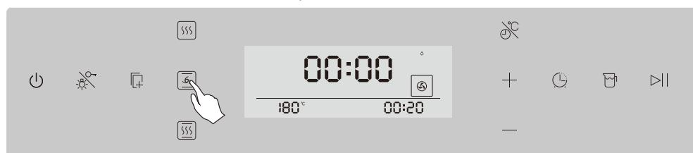
2. Once the work mode is selected, the default working time and temperature will be displayed. At this point: press the [Time/Temp] button to switch between adjusting the time or temperature (the selected one will flash). Use the [+] or [-] button to adjust the time or temperature: Short-press to adjust by 1 minute or 1°C. Long-press to continuously adjust.
